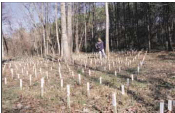
The effectiveness of preservatives at various retentions in different species is evaluated using test stakes. Arch monitors some 50,000 stakes in plots worldwide.
