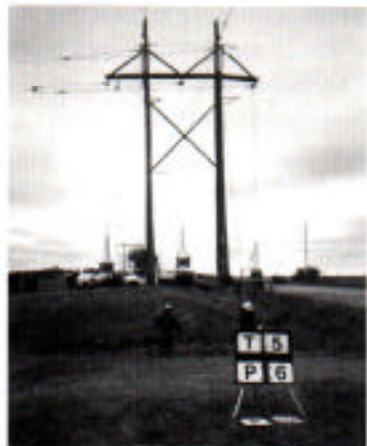
Full scale tests of 62-year old 115kV H-frames at Nebraska Public Power District (conducted by Engineering Data Management, Inc. and Hughes Brothers, Inc.)
