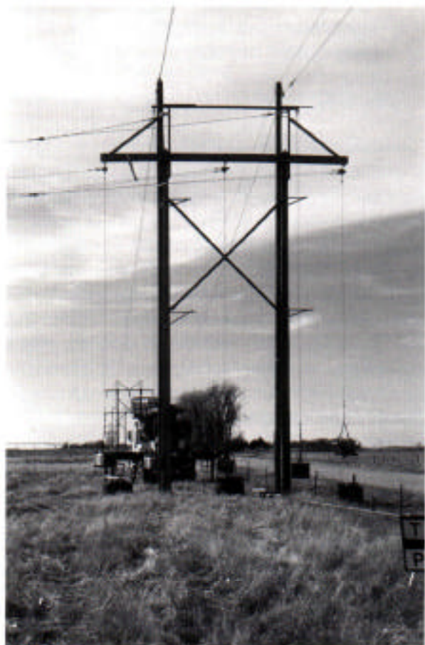
Full scale tests of 62-year old 115kV H-frames at Nebraska Public Power District (conducted by Engineering Data Management, Inc. and Hughes Brothers, Inc.)
