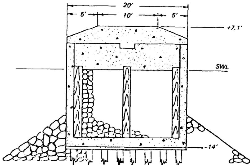
TYPICAL SECTION - NORTH BREAKWATER
