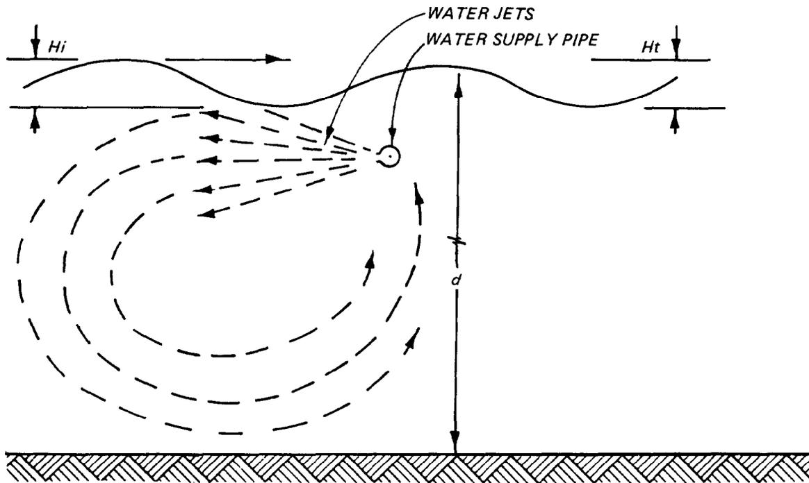
Figure 1-10. Conceptual sketch of the hydraulic breakwater
