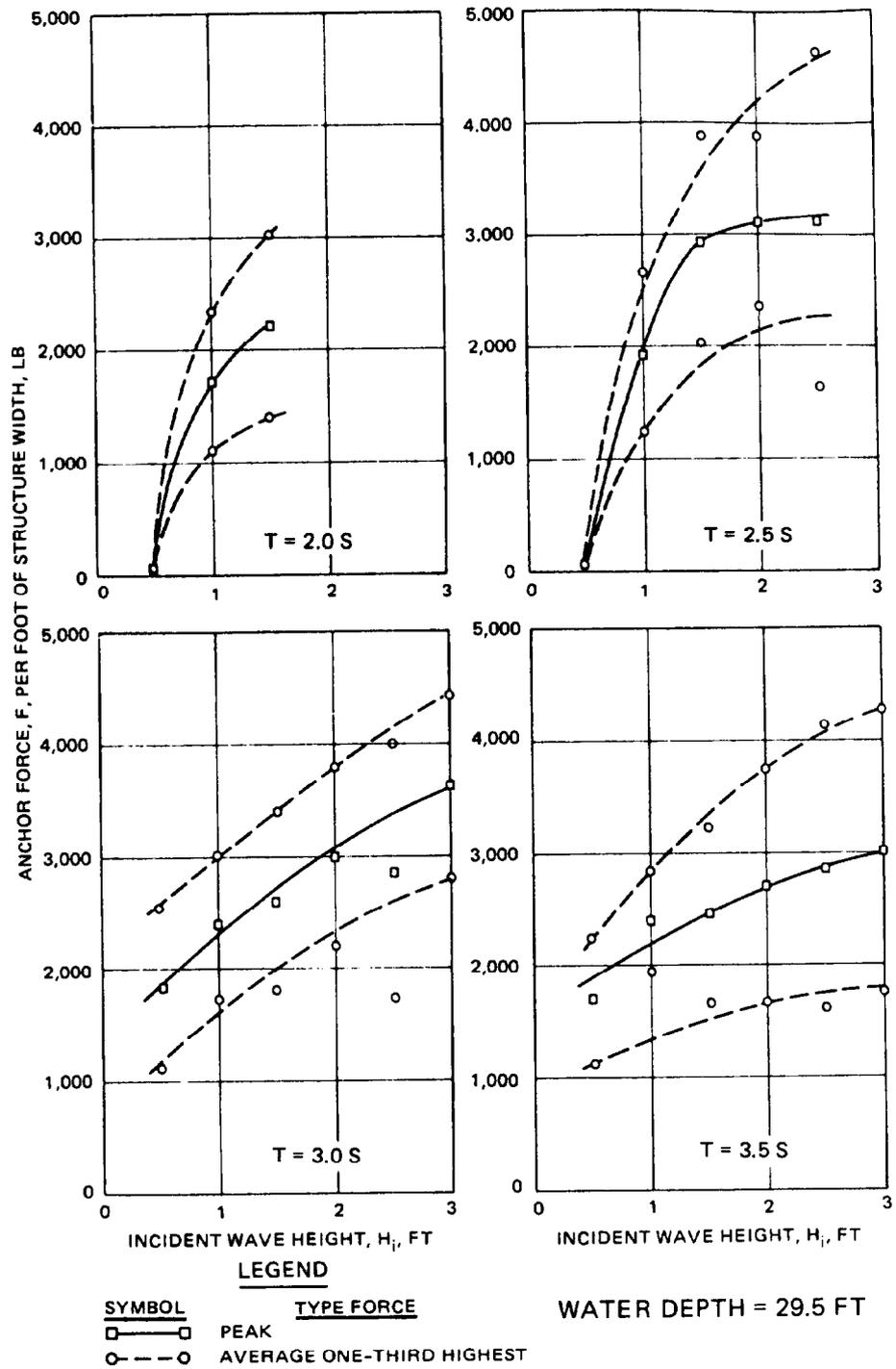
Figure 6-7. Anchor force test results for the pile mooring system, catamaran-type floating breakwater, Oak Harbor, Washington
