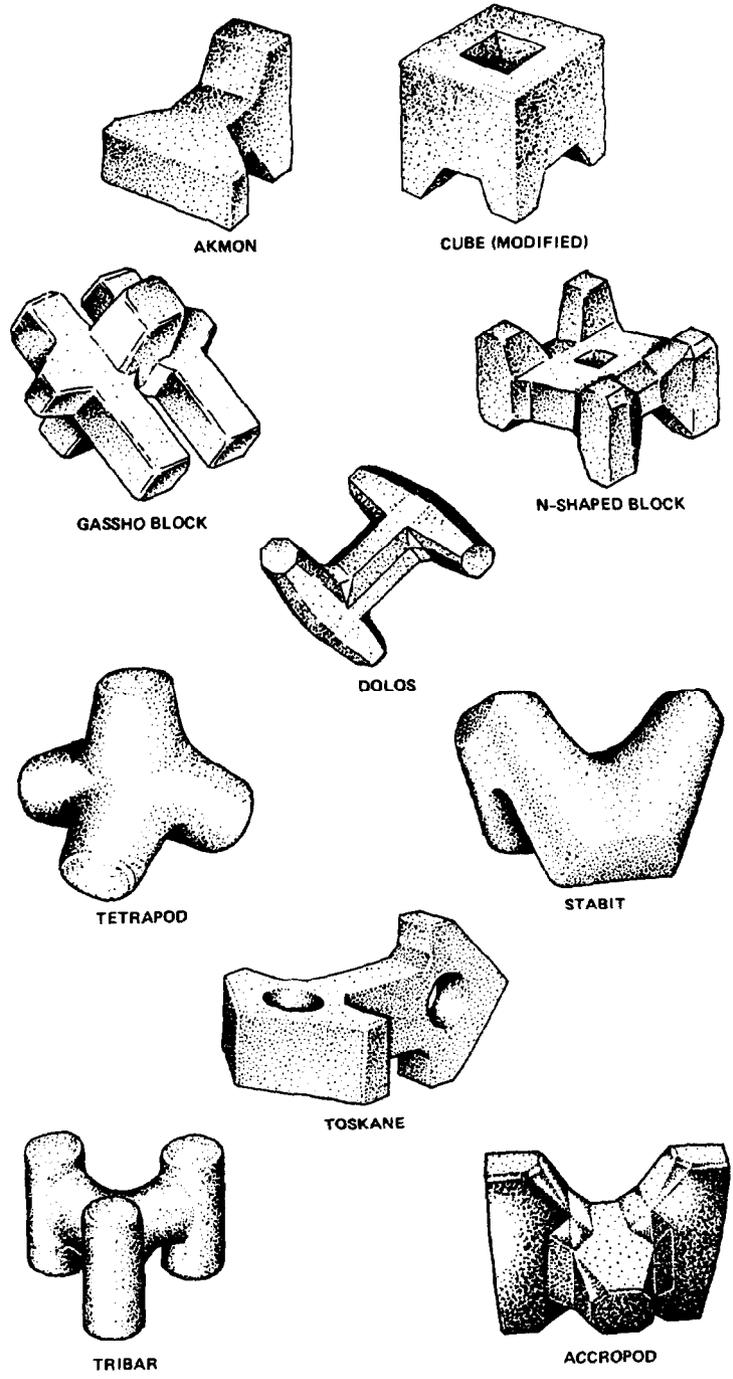
Figure 4-1. Concrete armor unit shapes
