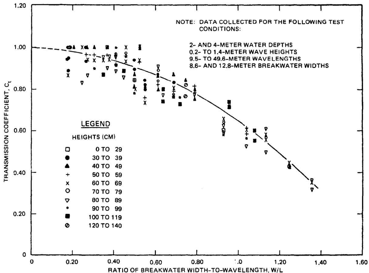
Figure 6-15. Design curve for determining width,  $W$ , of the Goodyear Tire and Rubber Company floating breakwater concept for various wave lengths,  $L$ , and allowable transmission coefficients,  $C_t$
