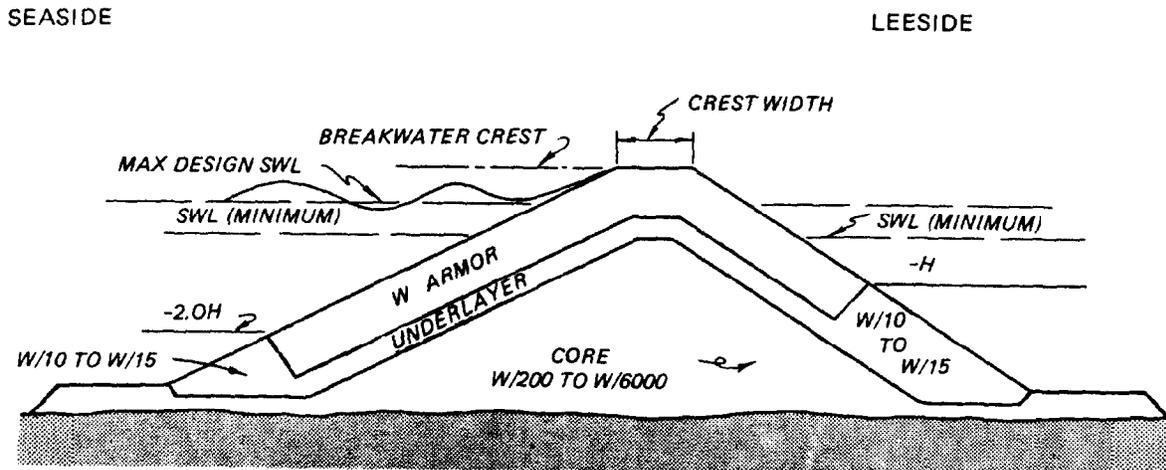
Figure 1-1. Typical rubble-mound section for seaside wave exposure
