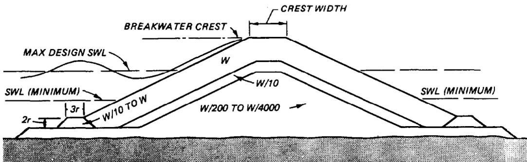
b. RUBBLE-MOUND SECTION FOR WAVE EXPOSURE FROM BOTH SIDES WITH MODERATE OVERTOPPING
