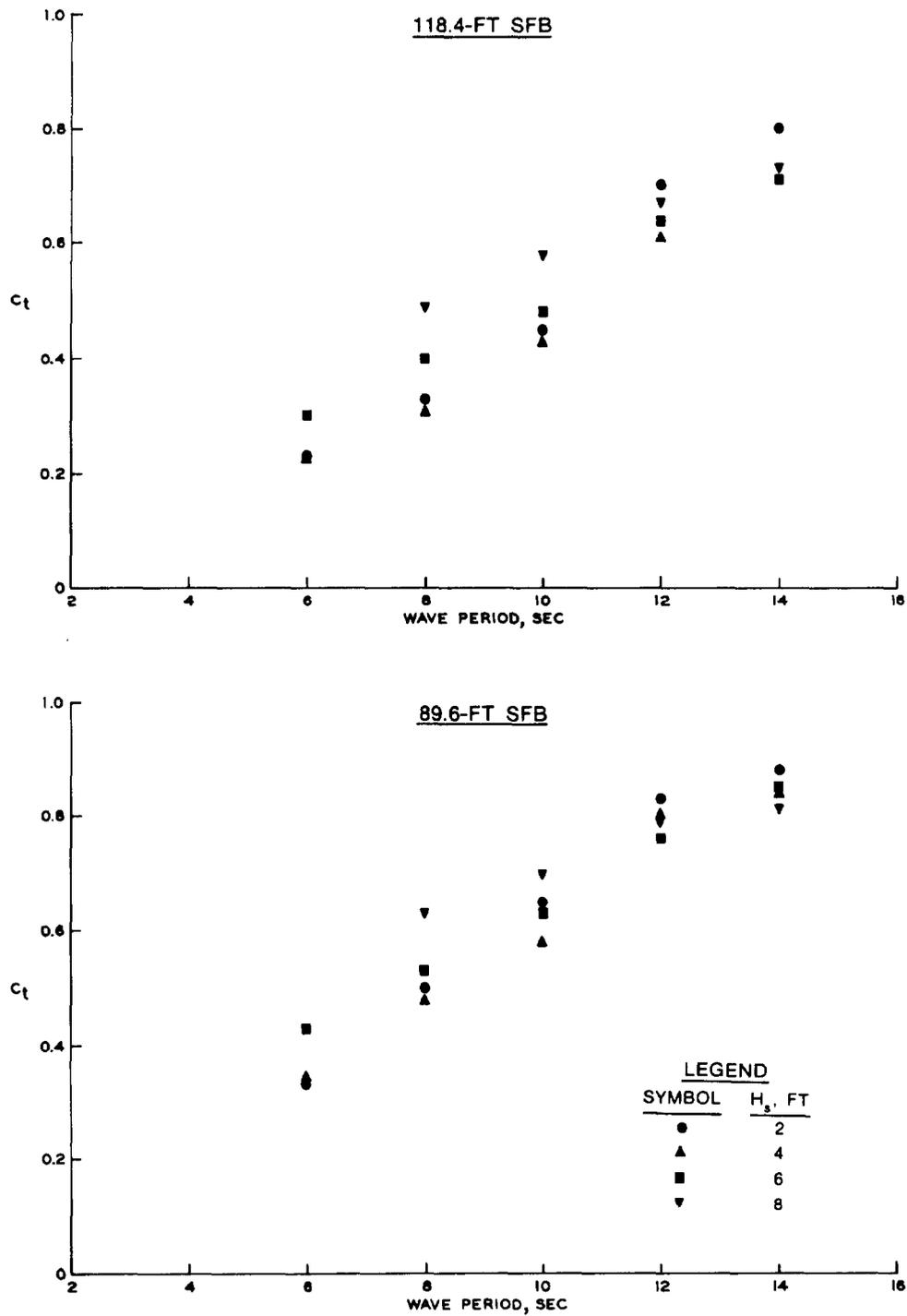
Figure 7-5. Wave attenuating capabilities of the SFB in an 18-foot water depth
