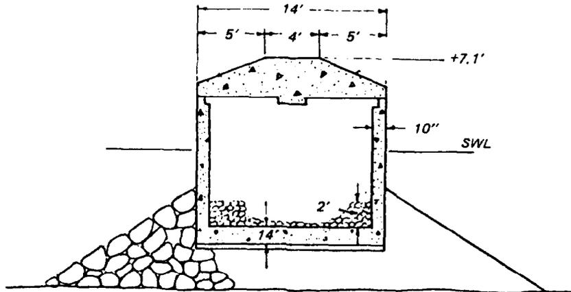
TYPICAL SECTION - NORTH AND SOUTH BREAKWATER
