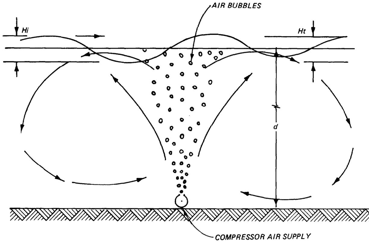
Figure 1-9. Conceptual sketch of the pneumatic breakwater
