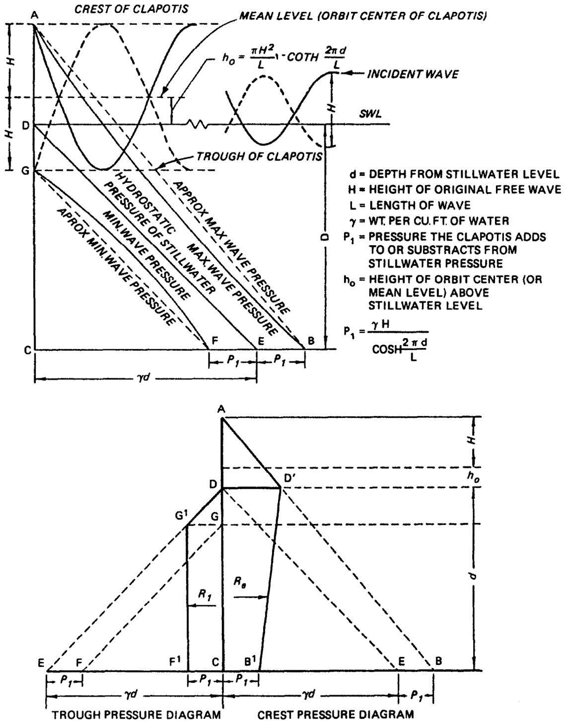
Figure 5-6. Nonbreaking wave loading on a vertical wall
