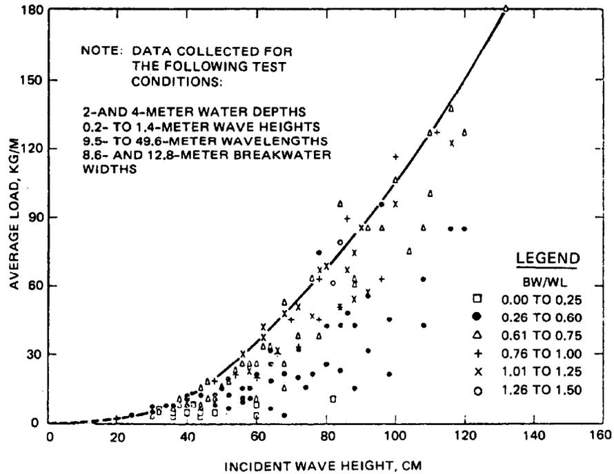
Figure 6-16. Design curves for predicting peak and average mooring forces for the Goodyear floating breakwater concept
