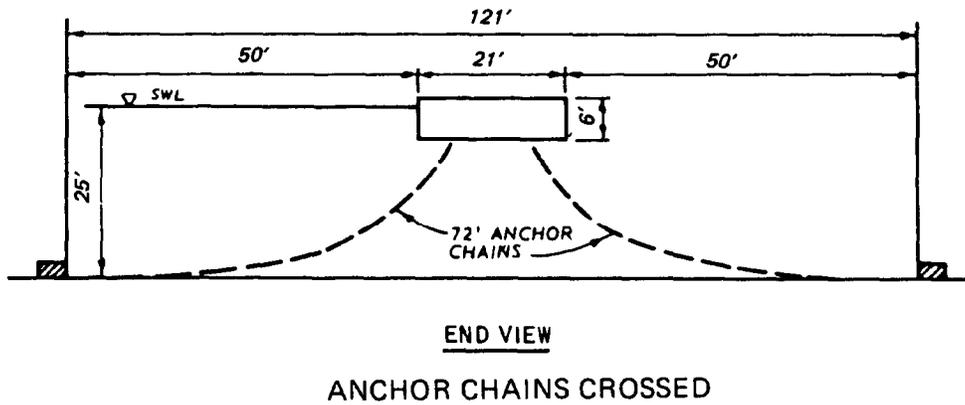
Figure 6-9. Mooring chain arrangement for Alaska-type floating breakwater evaluated in two-dimensional model tests for application at Olympia Harbor, Washington
