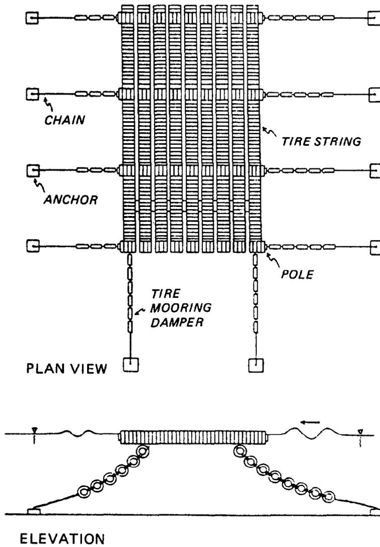
Figure 6-17. Schematic of wave-guard scrap-tire floating breakwater concept
