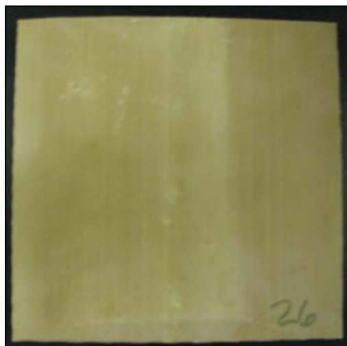
Figure 19. PVC 200-hour UV exposed specimen.
