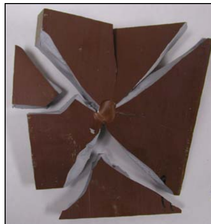
Figure 37. Intermediate-velocity impact damage in the PVC29 200-hour sample at the ballistic limit.
