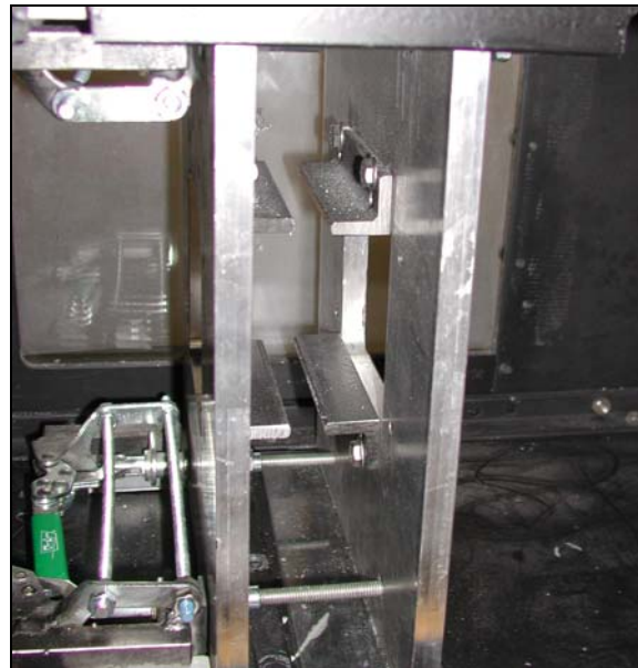
Figure 30. Specimen fixture for intermediate-velocity impact test.
