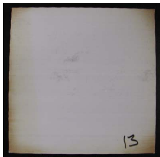
Figure 18. PVC 20-hour UV exposed specimen.
