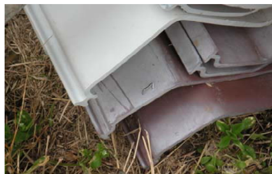
Figure 54b. Eight-year-old installations in Houma, Louisiana, Right bottom shows the eight-year-old unused sheet piles impacted with staple gun to show no cracking.
