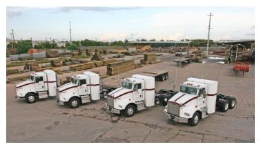
The new trucks are 2015 Kenworth T800's powered by Cummins Westport's new ISX12 G 400 engine, which is a 12 liter engine rated up to 400 horsepower and 1,450 lb-ft of torque. Building Products Plus is one of the first companies to have the 12 liter CNG-fueled trucks in operation.
