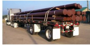
Poly coated pilings can double the life of treated pilings in water.
